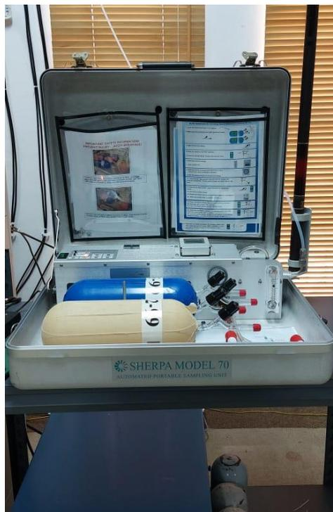
Gambar 1. *Air Kit Flask Sampler*
