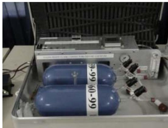
Gambar 14. *Airkit Flask Sampler*
