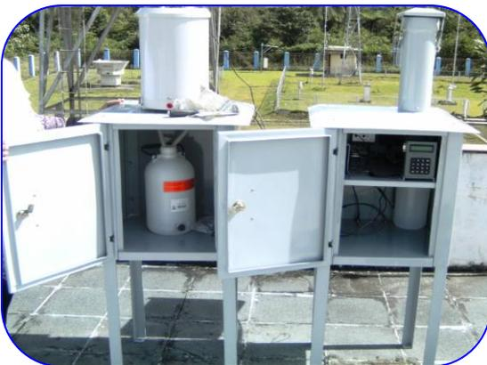
ARWS (Automatic Rain Water Sampler) tipe Automatic Precipitation Gauge\_GSM 200 series, dilengkapi modem GSM dan solar cell
