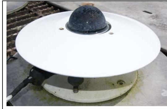
**Gambar 4.** Pyranometer RG8.
