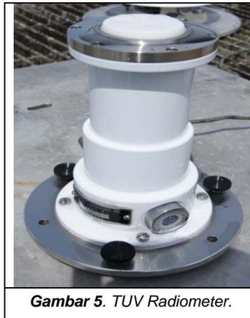
**Gambar 5.** TUV Radiometer.
