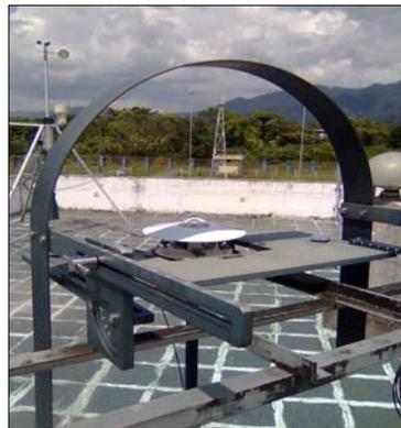
**Gambar 4.** *Eppley PSP dilengkapi Shadow Band*
